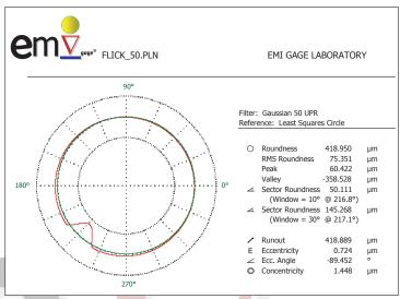
Typical roundness measurement of Flick detailing measured value for the calibrated Flick Standard. The operator can determine if the gage's gain is correct by simply looking at the measured value and comparing to the calibrated value.
