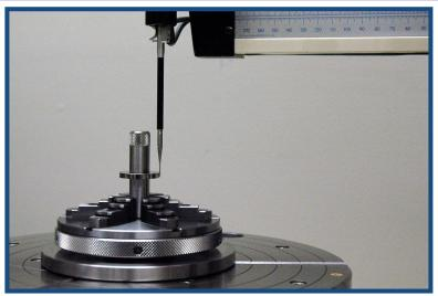
Above photo shows a dynamic verification using the Flick Standard. This procedure is a rapid verification of the probe gain and can be used daily to ensure proper system function.
